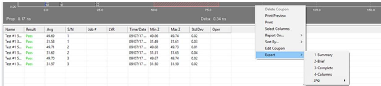
Right clicking on the DATALOG pane after some coupons have been saved , it will allow to export the entire results of tests. It is also possible to select what to export. In this case test data will be exported.
